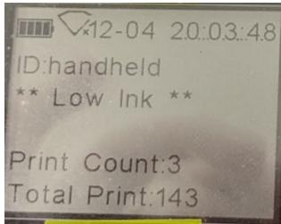
Press the "Back" button to turn on/off the scanner. Scan any supported barcode and swipe the device to print.
