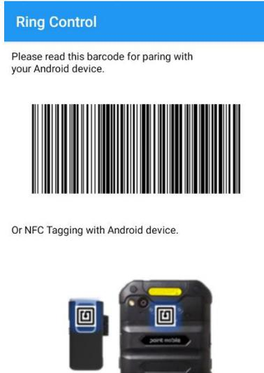
There are two ways for connection between ring scanner and host device, Scan-to-Pair and Tap-to-Pair. Choose more comfortable method.
